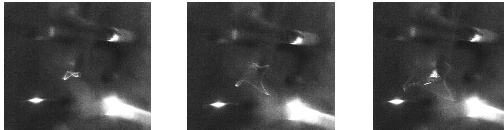
Figure 3. Images of the trajectory of the thread in the node (the first image), in the antinode without particles and in the antinode with charged particles. View from the end of the trap. In the lower right corner, a bright spot is visible due to the strong scattering of laser radiation on the trap electrode.
