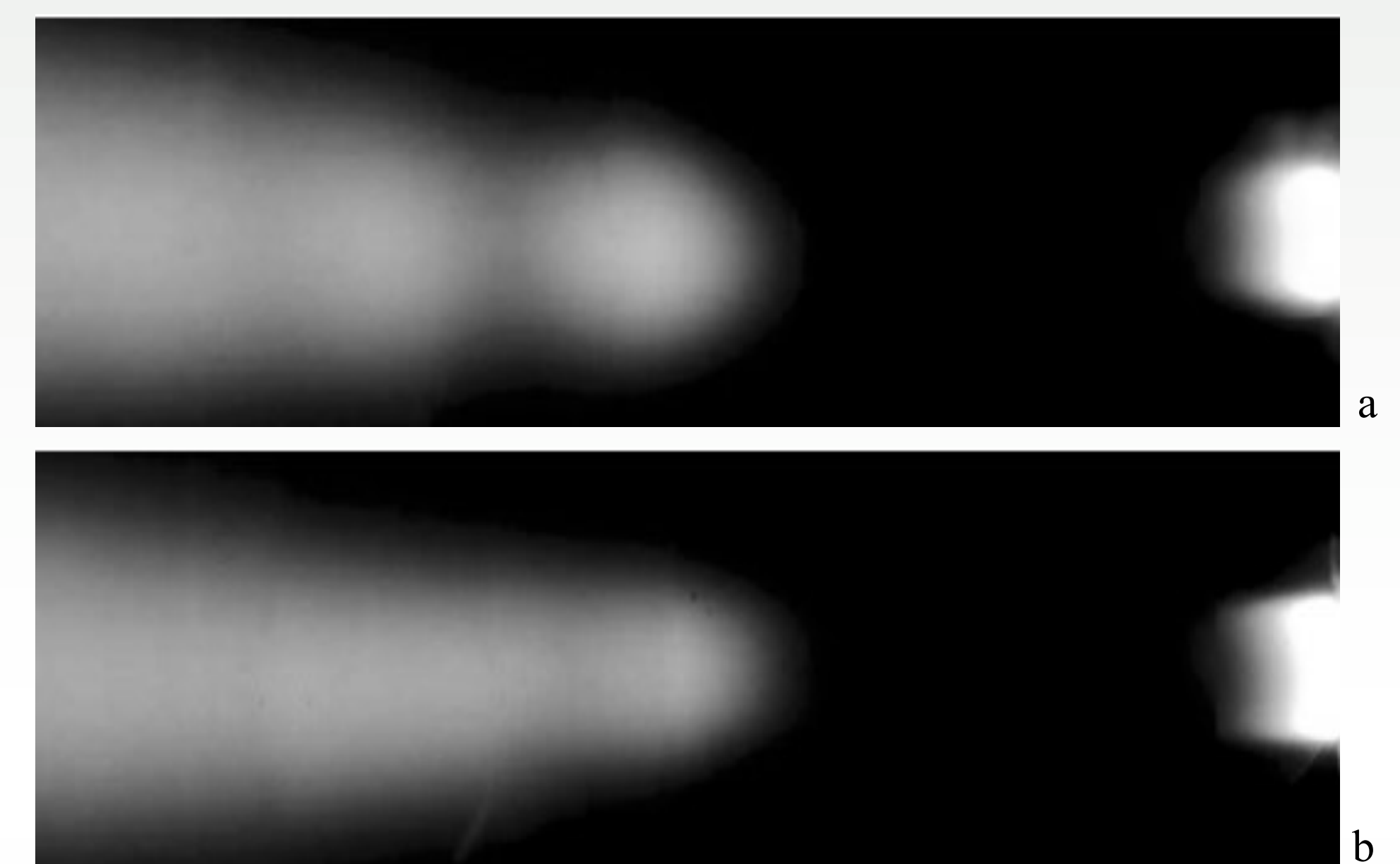
Fig.3. The images of the discharge at 1000 G (a) and 2700 G (b). At the right is the dielectric insert. Conditions: plasmaforming gas is neon, discharge current is 1.5 mA, gas pressure is 0.55 Torr, polydisperse quartz particles with main size 5-6mkm.
