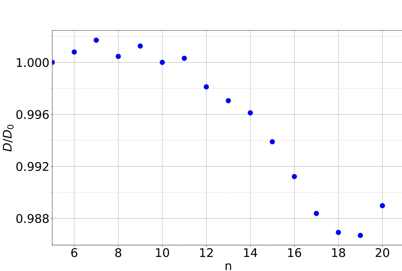
Diffusion coefficient in a melt with 65 % Nb on the of cut-off periods
