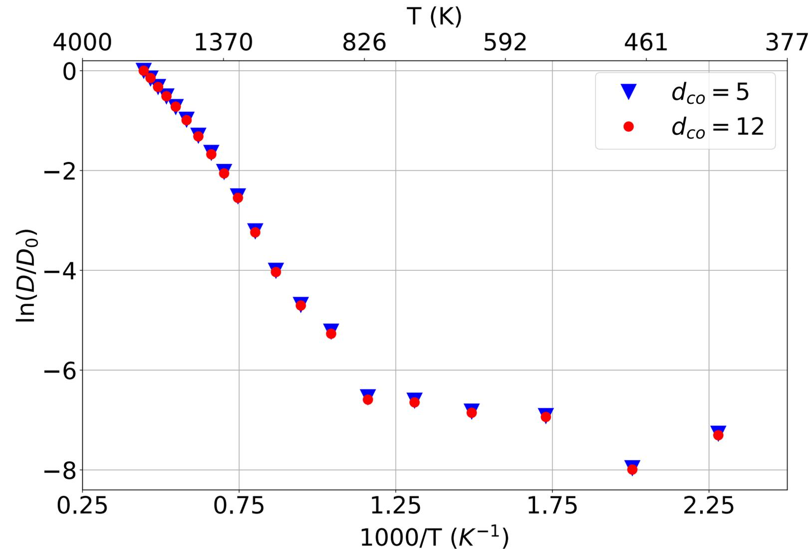
Diffusion coefficient on temperature for 65% Nb, cut-off distance 12 and 5 periods
