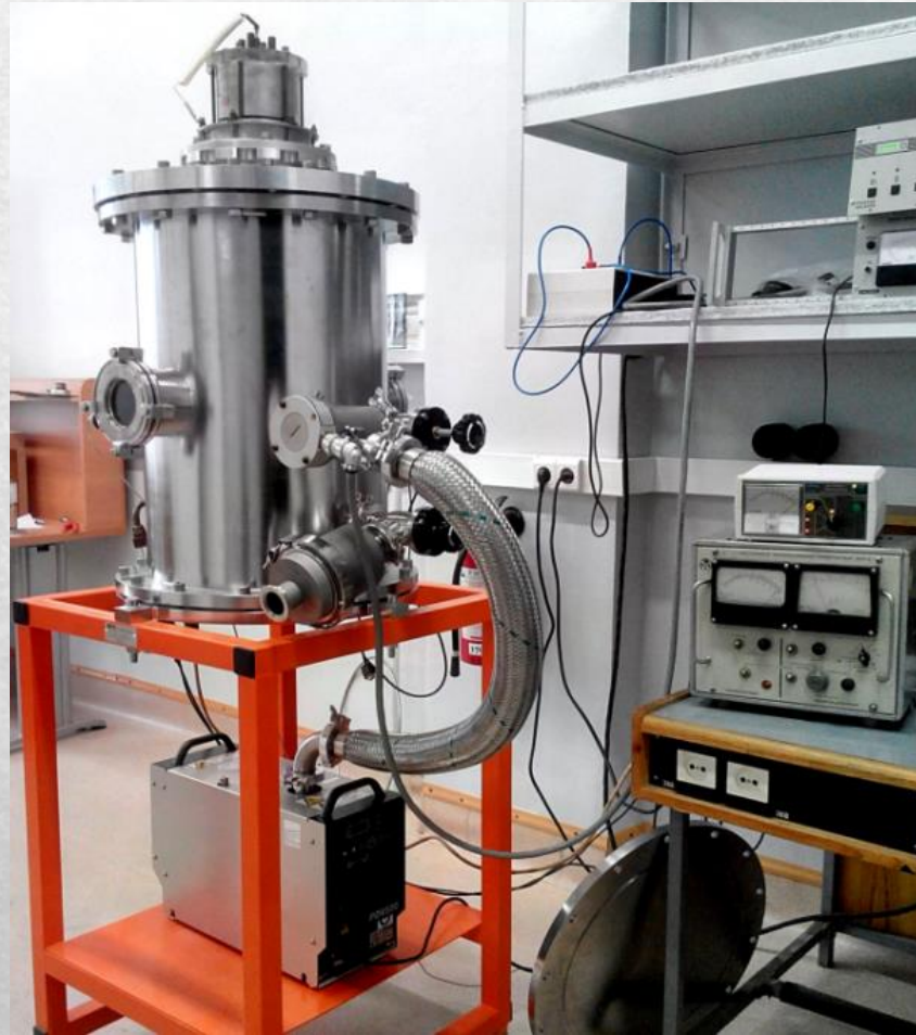
Vacuum chamber with dust injector (event with a frequency of 0.1 - 30 Hz)
