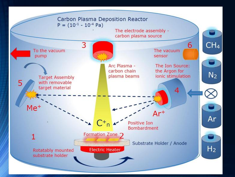
Schematic representation of the carbon pulse-plasma deposition reactor for growing of the carbyne-based nanostructures:
