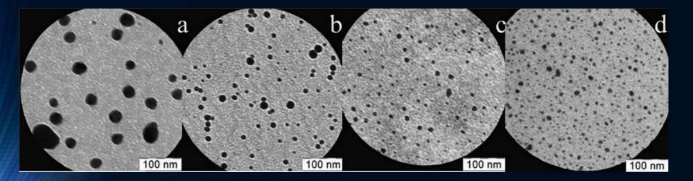
TEM images of the samples deposited at different ion assistance energies: (a) o eV, (b) 100 eV, (c) 200 eV, (d) 300 eV.
