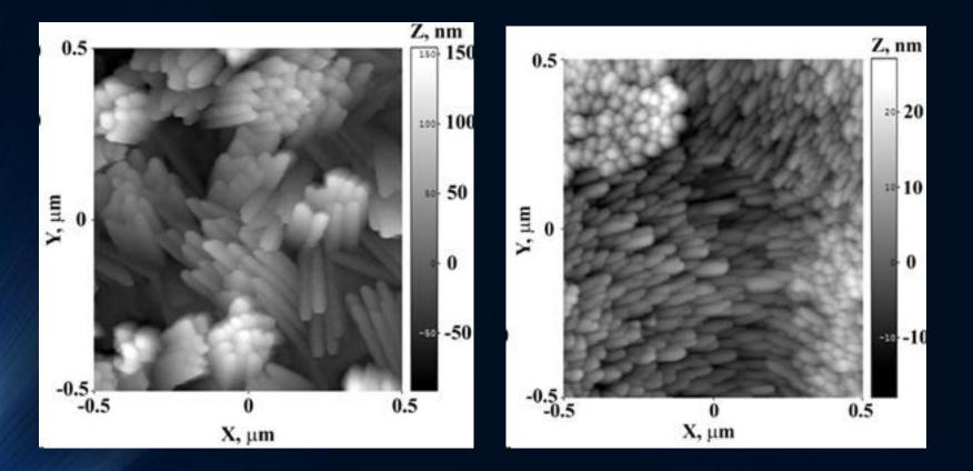
The atomic force microscopy (AFM) images of 150 nm thick Tellurium nanostructures, deposited at mechanical vibration frequencies of a) 50 Hz and b) 4 kHz.
