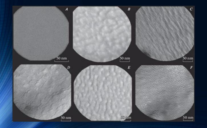
Transmission electron microscopy (TEM) patterns of samples obtained in different conditions: (A – o eV, B – 200 eV, C – 300 eV, D – 400 eV, E – 600 eV, F – 800 eV).
